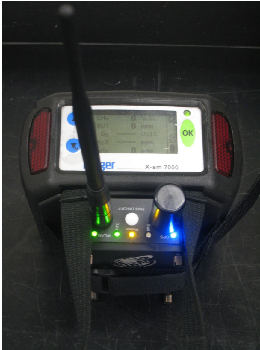
Figure 3. This photo shows the LINC connected to the Dräger® X-am 7000 multi-gas detector. The Dräger outputs its data via an infrared optical signal to the LINC, and the LINC transmits the data to the Life-line Gateway. Communication between the Dräger and LINC requires handshaking. As discussed in Figure 1, the Life-line Gateway sends the data it receives from the LINC to a laptop. The steady green light on the LINC labeled “Data” indicates that the data from the Dräger are successfully getting to the laptop. The steady green light labeled “WLAN” (Wireless Local Area Network”) indicates that communication to the Gateway is wireless. The orange light indicates that the LINC is powered on; the blue light, that it is receiving a GPS signal. If the battery were low, the light labeled “Batt” would be red.
