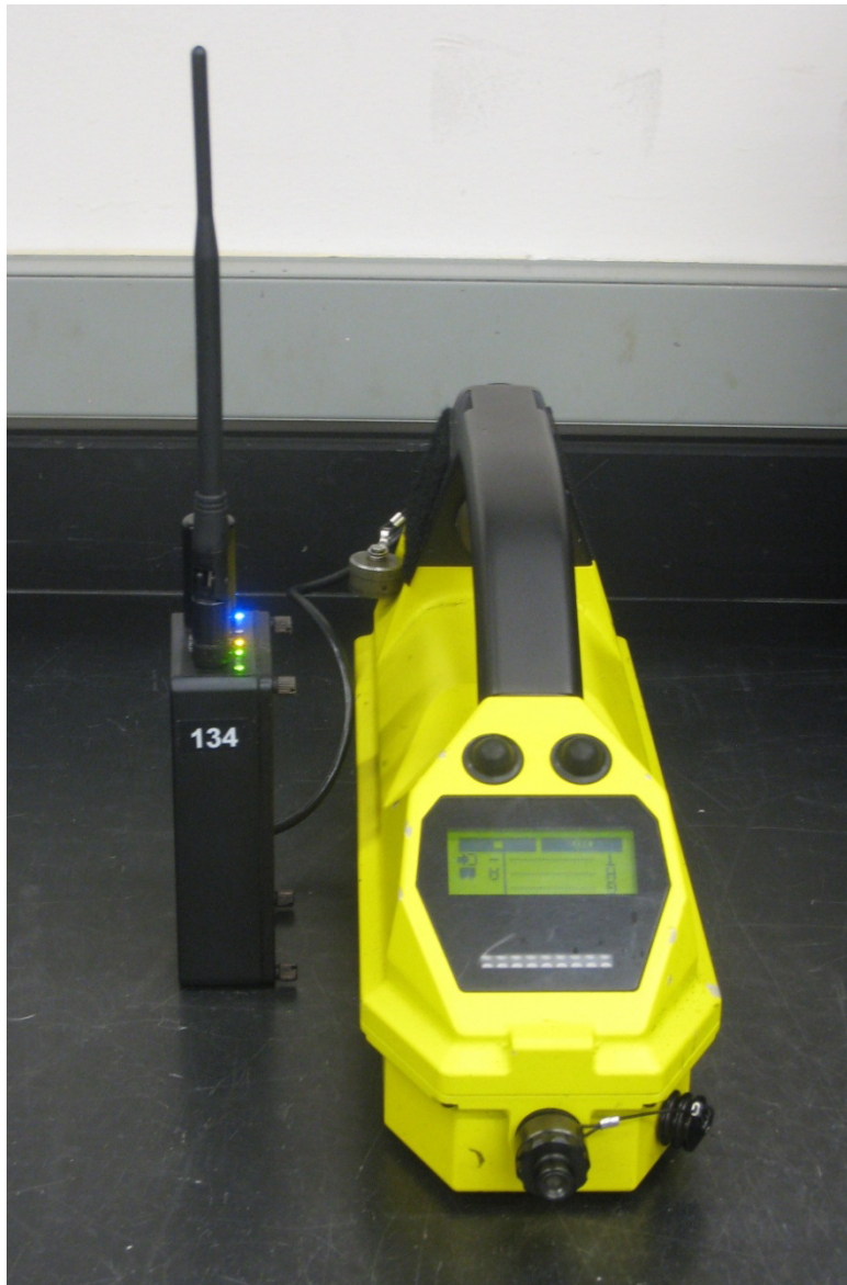
Figure 2. This photo shows the “Life-line Interoperable Network Communicator” (LINC) connected to the ion mobility spectrometer (IMS). The IMS outputs data as an RS-232 electrical signal. LINC receives the data and sends it to the Life-line Gateway. Communication between the IMS and LINC is initiated by handshaking. See Figure 3 for a close-up view of the lights on the LINC and their meanings.
