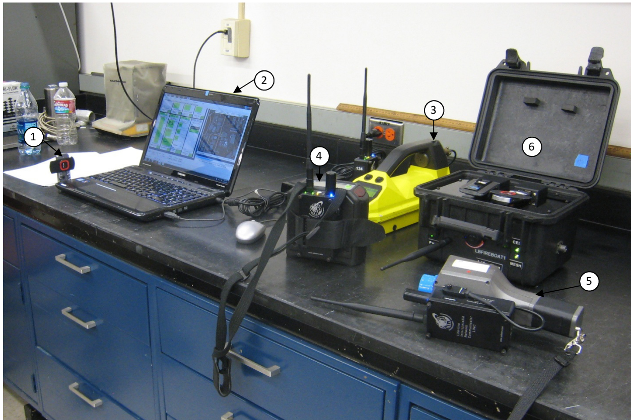
Figure 1. This is a photo of the test set-up. A Verizon 4G LTE cell card (1) was attached to a laptop (2), enabling the laptop to access the Internet wirelessly. The laptop used Life-line® software to read and display the output from three instruments, namely, a RAID® M100 ion mobility spectrometer (3) for detecting chemical warfare agents and toxic industrial chemicals, a Dräger® X-am 7000 multi-gas detector (4), and an ICX® (now FLIR®) identiFINDER (5) for detecting radiation sources and identifying the isotope emitting the radiation. Each of these instruments was connected a “Life-line Interoperable Network Communicator” (LINC), which wirelessly transmitted the data outputted from the instrument to the “Life-line Gateway” (6). The Life-line Gateway could be set to transmit the data received from the LINC’s directly to the laptop, or preferably, when a cell phone connection is available, the Life-line Gateway could be set to transmit data to a remote server via the cell phone connection. The laptop would then access the remote server on which the data are stored via the Internet.
